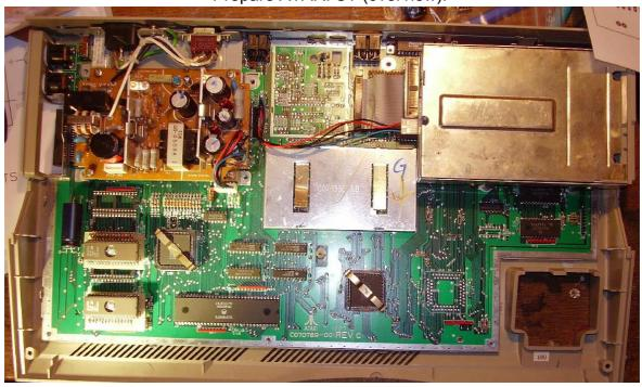
Setting the +5V supply to 5.15V using a Volt-meterTurn the variable resistor very slow while measuring voltage in the same time.
