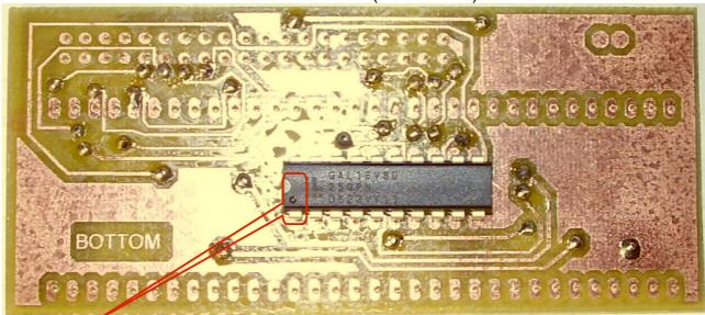
GAL PIN No. 1 (check mark before soldering GAL chip). Needs to be soldered on TOP-SIDE only. For PCB V1.4 don't use a socket to mount the GAL chip. There is very few space between CPU and interface.
