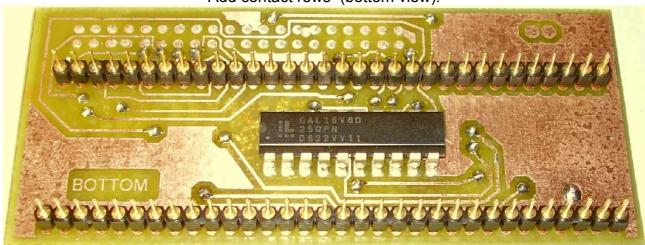
This contact rows have one thinner end. Plug the thinner end into the PCB and solder it on top side
