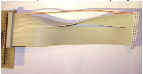
Pin 1 of the IDE connector is marked with a little triangle. The wires 1...2 and 19...40 must be connected without turning.
