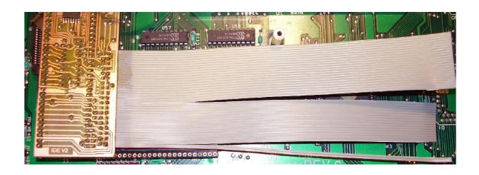
Mounting the IDE plug: Turn the cable part from wire No.3 to wire No.18 by 180 degree.
