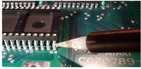
After soldering the CPU-socket check again for short circuit. If you are sure that everything is OK switch your ATARI ST on (without the IDE interface) and check function.
