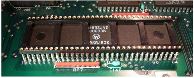
Solder each pin of CPU-socket with each pin of CPU. Prevent short circuit between pins:
